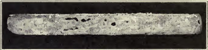
A RUSTED WATER PIPE
